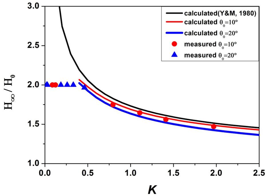
Figure 25. Comparison of calculated and measured normalized wave heights along the wall as a function of nonlinear parameter  $K$ . Black solid curve represents the wave height predicted by shock theory of Yue and Mei (1980), red and blue solid curves denote the calculated wave heights for  $\theta_0 = 10^\circ$  and  $20^\circ$ , respectively. Symbols are measured data.
