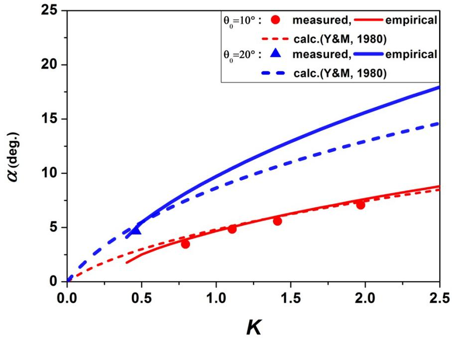
Figure 28. Comparison of calculated and measured stem angle  $\alpha$  as a function of nonlinear parameter  $K$ . Dashed curves represent the calculated values using Yue and Mei (1980), solid curves are the calculated values using the present empirical formula, symbols are measured data. Red and blue colors are for  $\theta_0 = 10^\circ$  and  $20^\circ$ , respectively.
