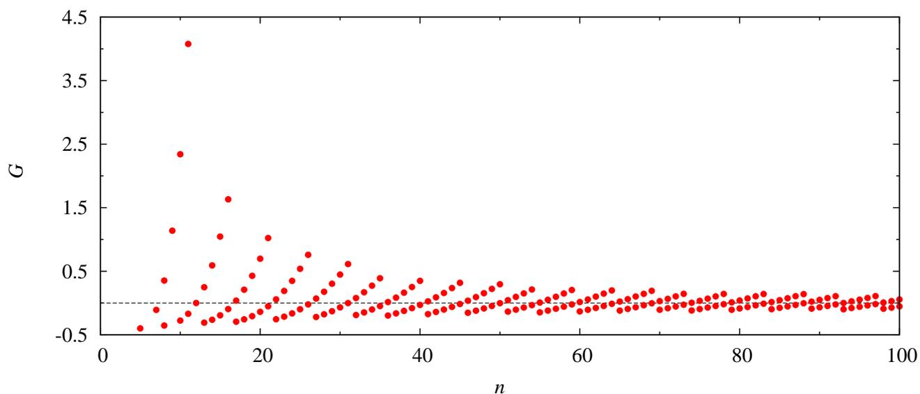
**Figure 10.**  $G$ -coordinates of double-Hopf points as a function of  $n$ . Only those double-Hopf points are shown which destabilize the equilibrium  $x_F$ . For large values of  $n$  the double-Hopf bifurcations are close to the  $F$ -axis in the  $(F, G)$ -plane, which means that these points are likely to affect the dynamics of the Lorenz-96 model for  $G = 0$ .
