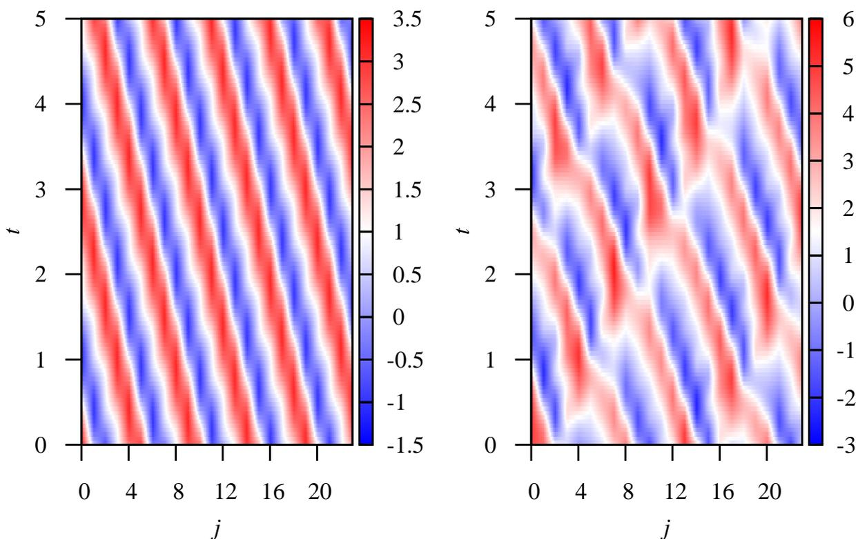
**Figure 1.** Hovmöller diagrams of a periodic attractor (left,  $F = 2.75$ ) and a chaotic attractor (right,  $F = 3.85$ ) in the Lorenz-96 model for  $n = 24$ . The value of  $x_j(t)$  is plotted as a function of  $t$  and  $j$ . For visualization purposes linear interpolation between  $x_j$  and  $x_{j+1}$  has been applied in order to make the diagram continuous in the variable  $j$ .
