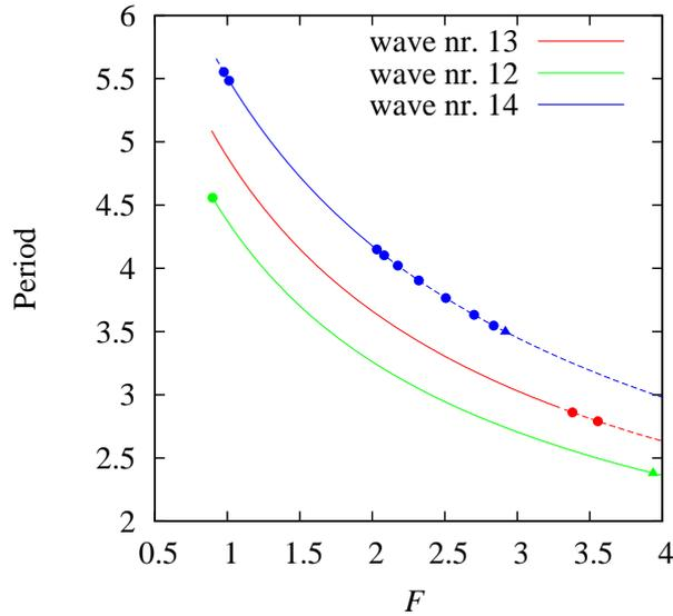
**Figure 12.** As Figure 11, but for  $n = 60$ . For  $1.01 < F < 2.03$  three stable periodic orbits coexist. The Hopf bifurcations generating the waves with wave numbers 13, 12, 14 occur at respectively  $F = 0.891$ ,  $F = 0.894$ , and  $F = 0.923$ .
