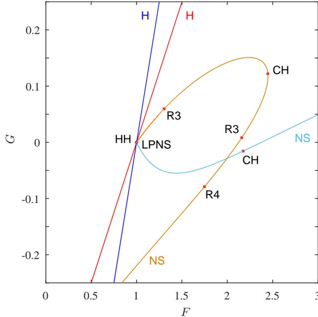
**Figure 8.** Bifurcation diagram of the 2-parameter system (14) in the  $(F, G)$ -plane for  $n = 12$ . A double-Hopf bifurcation point is located at the point  $(F, G) = (1, 0)$  due to the intersection of two Hopf bifurcation lines. From this codimension-2 point two Neimark-Sacker bifurcation curves emanate which bound a “lobe-shaped” region in which two periodic attractors coexist.
