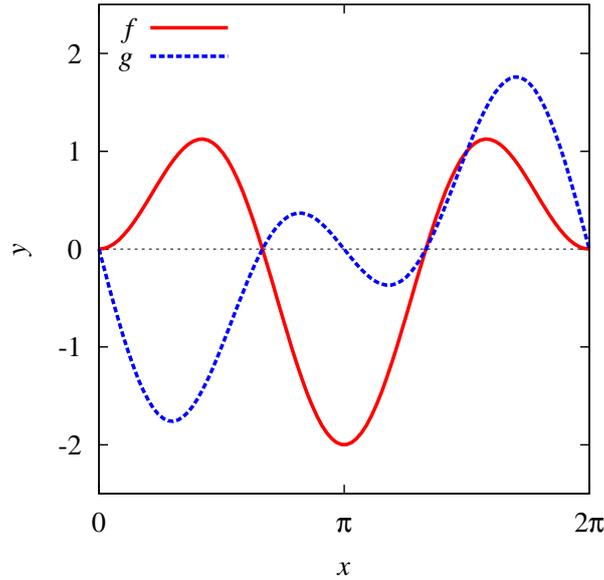
**Figure 3.** Graphs of the functions  $f$  and  $g$  as defined in Eq. (5). The eigenvalues of the equilibrium  $\mathbf{x}_F = (F, \dots, F)$  are given by  $\lambda_j = -1 + Ff(2\pi j/n) + Fg(2\pi j/n)i$  for  $j = 0, \dots, n-1$ . The shapes of the graphs of  $f$  and  $g$  imply that the equilibrium  $\mathbf{x}_F$  can only lose stability through either a Hopf or a double-Hopf bifurcation for  $F > 0$ .
