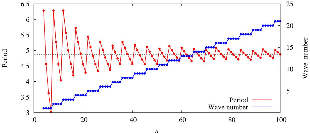
**Figure 4.** As the equilibrium  $x_F = (F, \dots, F)$  loses stability through a (double-)Hopf bifurcation for  $F > 0$  a periodic attractor is born which represents a traveling wave. The spatial wave number increases linearly with  $n$ , whereas the period tends to a finite limit.
