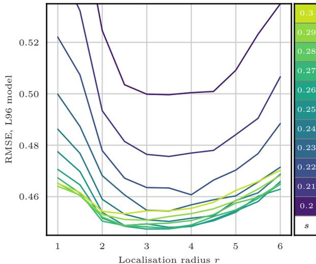
**Figure 5.** RMSE as a function of the localisation radius  $r$  for the S(IR) $\times$ R algorithm with  $N_e = 10$  particles,  $N_b = 40$  blocks of size 1 grid point and no integration jitter ( $q = 0$ ). For each  $r$ , several values for the regularisation jitter  $s$  are tested as shown by the colour scale.
