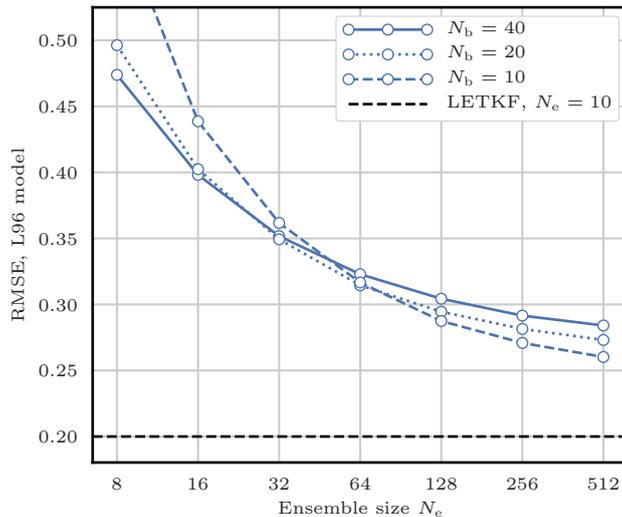
**Figure 8.** RMSE as a function of the ensemble size  $N_e$  for the  $S(\text{IR})^{\times R}$  algorithm with respectively  $N_b = 40, 20, 10$  blocks of size 1, 2, 4 grid points.
