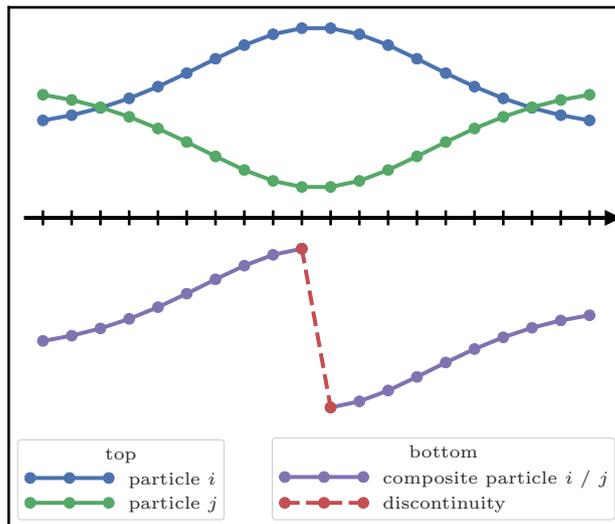
**Figure 3.** Example of one-dimensional concatenation of particle  $i$  on the left and particle  $j$  on the right. Top: the prior particles  $i$  and  $j$ . Bottom: the composite particle, concatenation of  $i$  and  $j$ . In this situation, a large unphysical discontinuity appears at the boundary.
