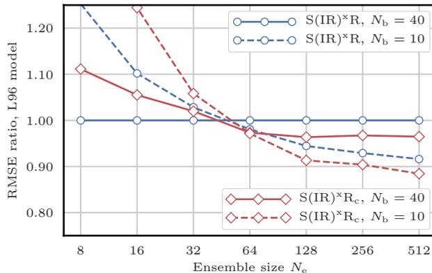
**Figure 11.** RMSE as a function of the ensemble size  $N_e$  for the  $S(IR)^xR$  and the  $S(IR)^xR_c$  algorithms with respectively  $N_b = 40, 10$  blocks of size 1, 4 grid points. The scores are displayed in units of the RMSE of the  $S(IR)^xR$  algorithm with  $N_b = 40$  blocks of size 1 grid point.
