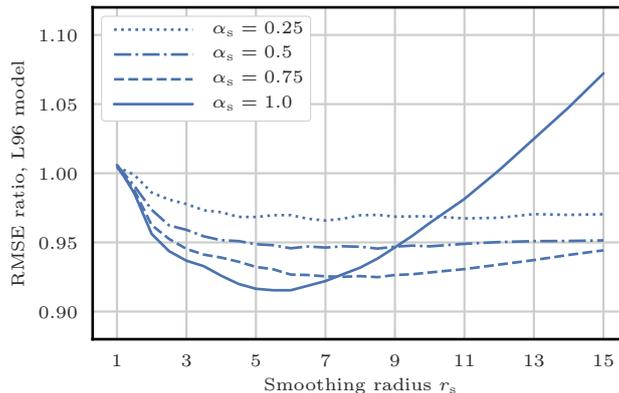
**Figure 12.** RMSE as a function of the smoothing radius  $r_s$  for the  $S(\text{IR})^x\text{S}_{\text{PMR}}$  algorithms with  $N_e = 16$  particles and  $N_b = 40$  blocks of size 1 grid point for several values of the smoothing strength  $\alpha_s$ . The scores are displayed in units of the RMSE of the  $S(\text{IR})^x\text{R}$  algorithm with  $N_e = 16$  particles and  $N_b = 40$  blocks of size 1 grid point.
