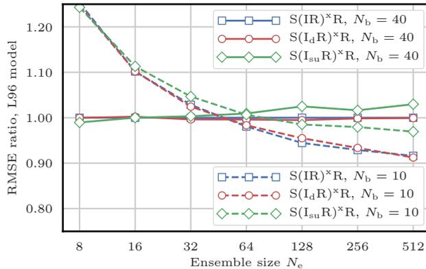
**Figure 10.** RMSE as a function of the ensemble size  $N_e$  for the  $S(IR)^{xR}$ , the  $S(IR_d)^{xR}$  and the the  $S(IR_{su})^{xR}$  algorithms with respectively  $N_b = 40, 10$  blocks of size 1, 4 grid points. The scores are displayed in units of the RMSE of the  $S(IR)^{xR}$  algorithm with  $N_b = 40$  blocks of size 1 grid point.
