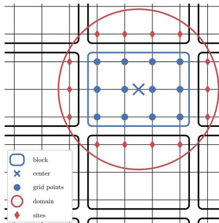
**Figure 2.** Example of geometry in the SBD localisation formalism for a two-dimensional space. The focus is on the block in the middle which gathers 12 grid points. The local domain is circumscribed by a circle around the block center with potential observation sites outside the block.
